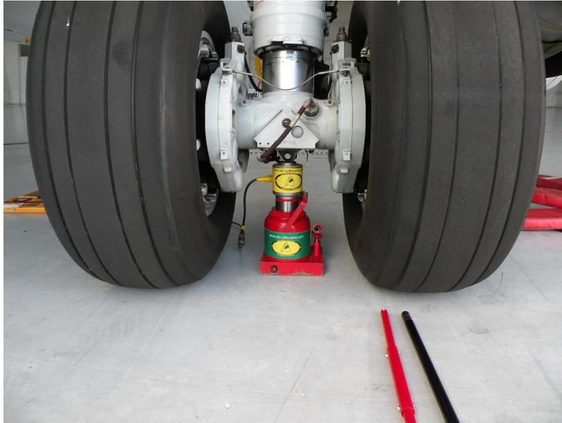
If more than one inch clearance is over the top jack adapter will be required as shown below:
