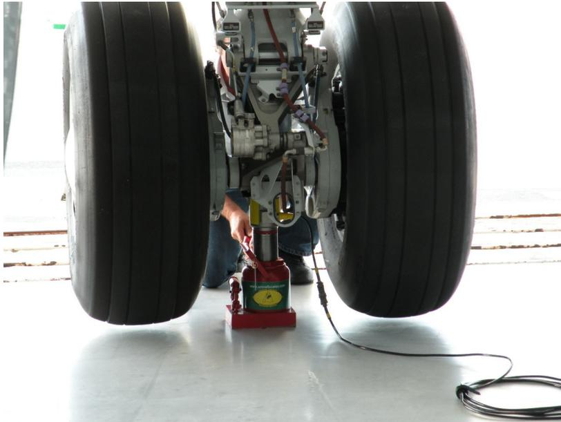
If the jacks run out of lift prior to clearing the ground then jack adapters should have been used. In some conditions, ½ inch shim plates can be placed under the tires and or jacks to shim accordingly to obtain the proper lift.
