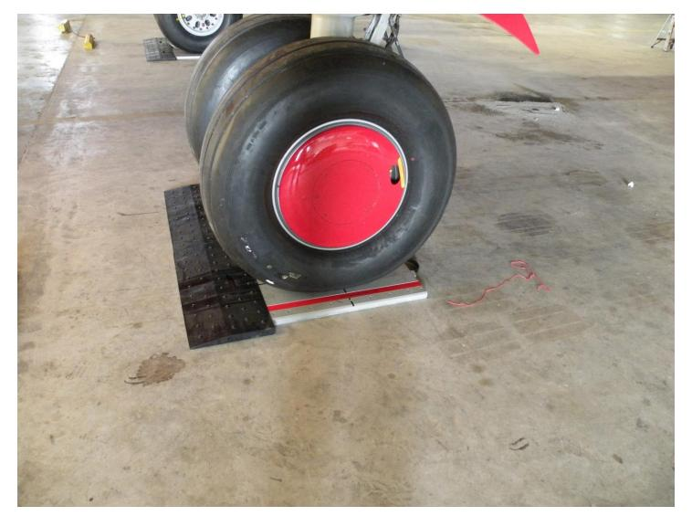
Here you can see the full contact patch and width requirement for large aircraft tires. It is critical to understand that this system will not necessary fit every type of aircraft. Always consider that the platforms are rated at 30,000 lbs., the tire must be inside the weighing area and your measurements are critical in your determination for use. All loads must be in the center of the platform to ensure that your weighing is accurate.
