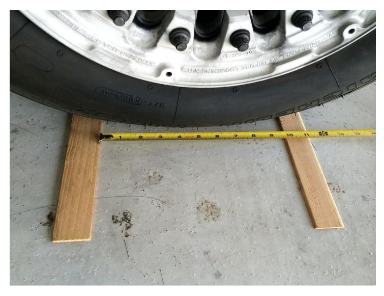
Here we show a tire being measured for fit. We check the foot print in two ways, length as shown and width. Take two paint stir sticks and lay them under the tire fore and aft as shown. Your measurement must be less than that of the live weighing area of 12.5 inches
